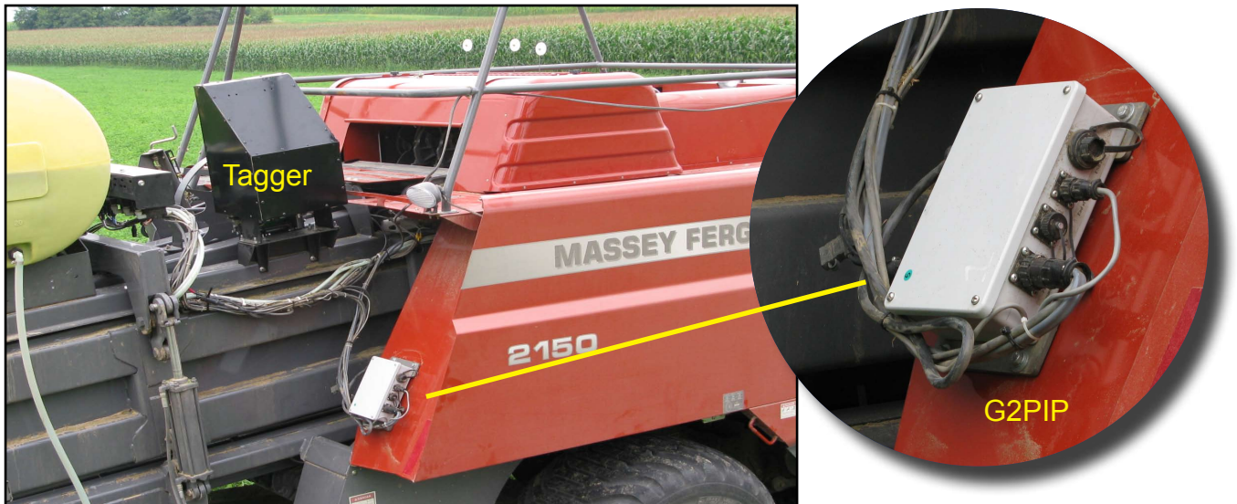
HayBoss G2 shown with new G2 Precision Information Processor and Individual Bale Identification Expansion "Tagger" Module
